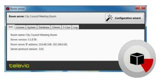
The Room Server application is the beating heart of the CoCon environment. It is responsible for the communication with the central conference unit and is typically installed on a machine located in a server room. As a result, it enjoys the same power advantages as the central unit itself.
